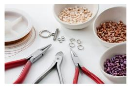
1 m of 0.38 mm nylon copper binding wire; 1x ø 15 mm American fastening; 2x ø 8 mm rings, 0.8 mm thick; 2x ø 6 mm rings, 1 mm thick; 4x ø 5 mm rings snipping pliers, 2x flat nose, round or needle nose pliers; a soft A4 pad
